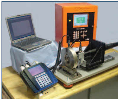
Torque Tension Test System
