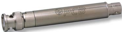
Model 426B02 In-line “A-weighting” Filter
