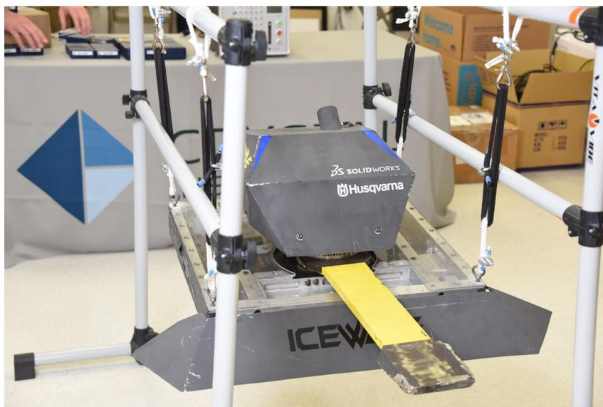
Icewave has an overall record of seven wins and six losses. Marc DeVidts, Icewave creator and team lead, believes some of the losses may have been due to the blade not impacting opponents effectively. Because of the power behind Icewave, some of these losses can be attributed to self-inflicted damage from its own rotating horizontal blade. The modal testing will be used to help increase striking effectiveness.
