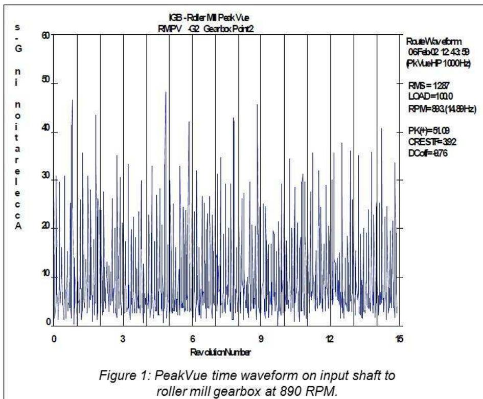
Each of the 1,024 data points in the PeakVue™ time data block contains the absolute peak value that was detected over each sequential 0.977 msec time increment. For the entire time data block (that includes fifteen revs of the shaft), the peak value is 51g's, which is the parameter recommended for trending when carrying out PeakVue™ analysis. The trended values for this measurement point (input on roller mill gearbox) over a 300 day time period are presented in Figure 2.
