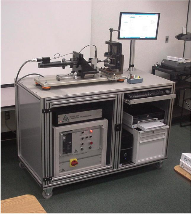
**Portable Fastener Test System**
