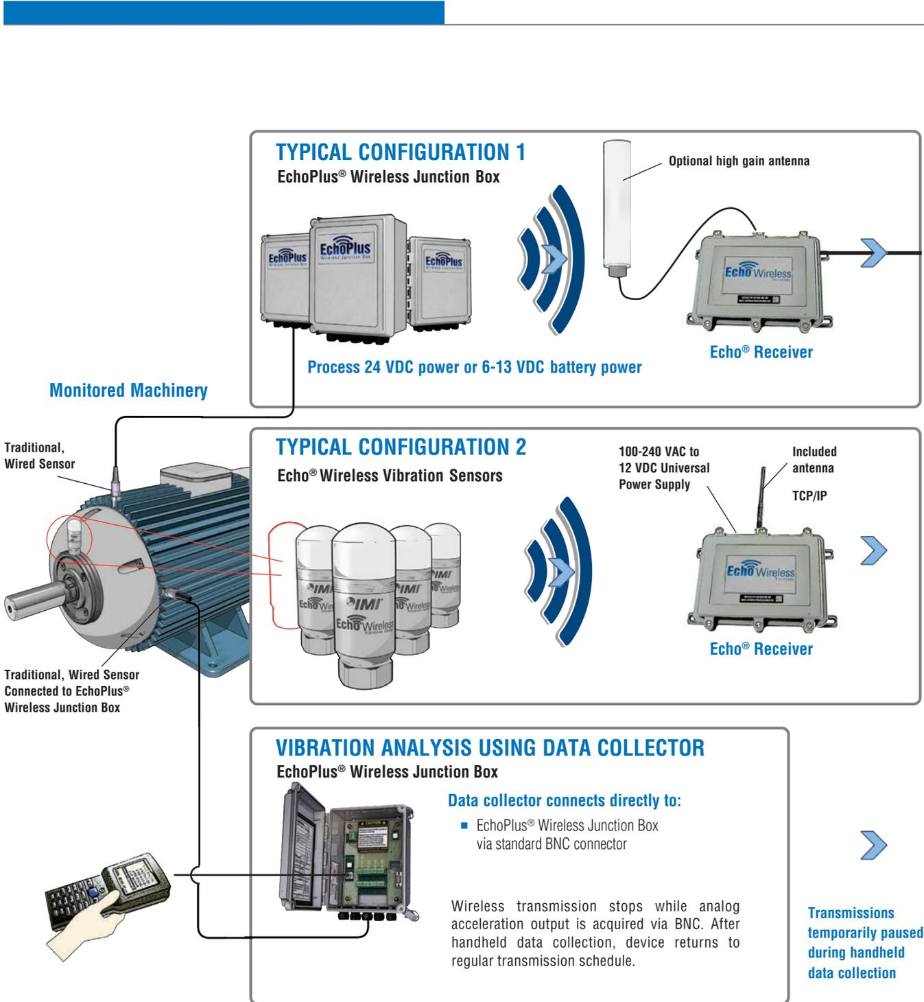
The Echo® Wireless Vibration Monitoring System is simple in design, easy to install, cost-effective and flexible in configuration. With over 400 points per receiver, the system can monitor over 3,500 points even within the same RF coverage area. Outside the same coverage area, the number is even higher. Stand-alone Echo® Sensors and EchoPlus® Junction Boxes can be mixed and matched as desired.
