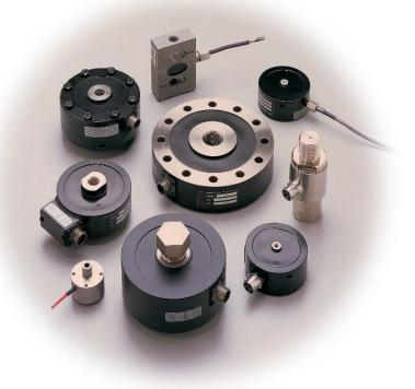
PCB Piezotronics offers strain gage load cells for precision measurement requirements. A variety of configurations are available, which include: low profile, fatigue rated, rod style, and S-beam types.
