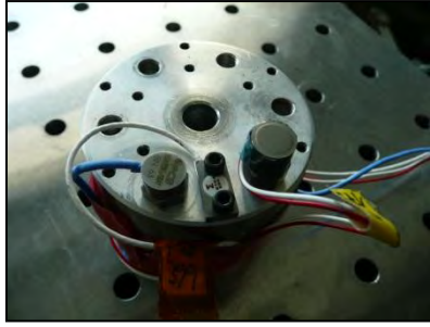
Figure 28a: Test arrangement of shock sensors.
