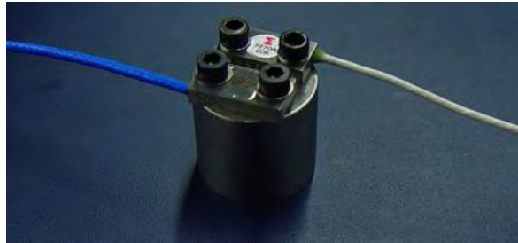
Figure 14: PCB and Legacy Shock Accelerometer on Breakaway Fixture
