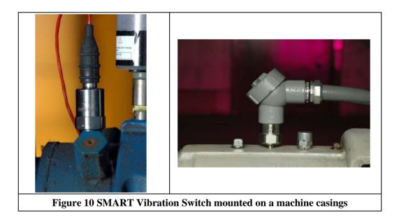
The Smart Vibration Switch should be mounted like an industrial accelerometer in the horizontal direction on the motor and fan bearings at the location of highest load for the best performance. The Smart Vibration Switch operates over two wires and installs in series with a load and its power source to form a loop. A typical connection schematic of a SMART Switch is shown in Figure 11 [7]
