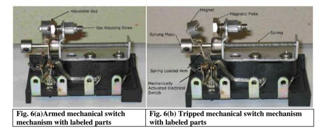
The gap between the magnet and magnetic plate can be adjusted by an external screw adjustment to increase or decrease the magnetic force holding the spring loaded arm in an armed position. Unfortunately, not all mechanical switches have the same maximum gap or force adjustment per turn. Some switches that this author looked at had a maximum gap of only 4.3 to 5.1 mm beyond which the magnetic force is not strong enough to overcome the spring force. Other mechanical switches had
