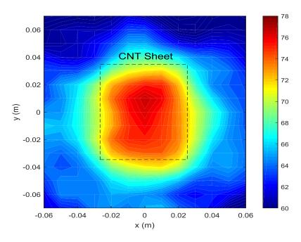
SPL (dB) distribution on Source Frequency=2000 Hz
