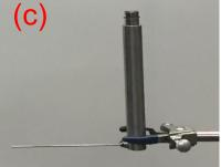
Test setup shown on lab bench. Actual test took place in a fully anechoic chamber at Michigan Tech. a) Photograph of the NAH test setup showing the moving probe microphone mounted to the vertical and horizontal translation stage, the stationary probe microphone mounted to the base plate, the CNT speaker b) Top view showing the probe microphones and the distance from CNT sheet (5mm). c) PCB model 377B26 probe microphone.
