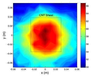
Measured SPL (dB) distribution Frequency=2000 Hz
