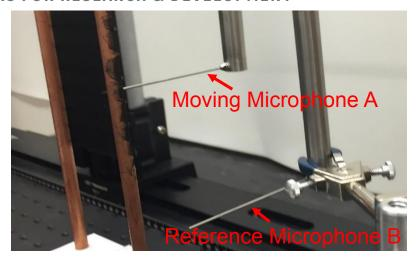
Photograph of the reference and moving probe microphone
