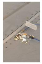
(b) F-16 left wing collocated strain sensor and accelerometer
