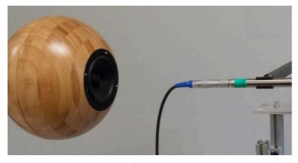
Figure 6: Speaker arranged on axis of the microphones during pressure calibration.
