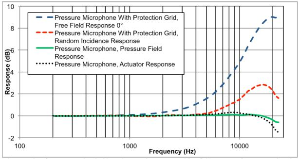
Figure 1: Plot of pressure, random incident, electrostatic actuator, and free field response of a pressure microphone.
