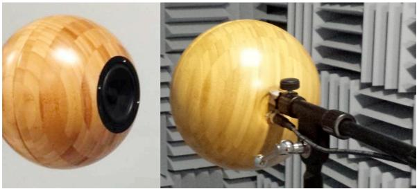
Figure 2: Spherical speaker front and back view.
