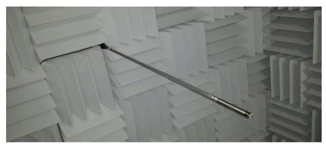
Figure 4: Wall mounted rod fixture for free field calibration.
