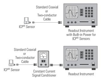
Figure 3. Typical ICP® Sensor Systems
