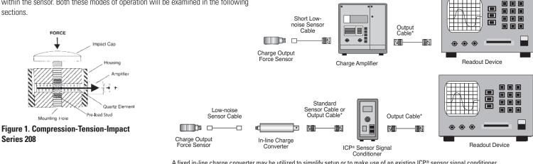
A fixed in-line charge converter may be utilized to simplify setup or to make use of an existing ICP® sensor signal conditioner
