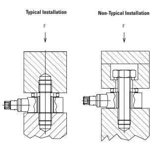
Figure 8. Force Ring Sensor Installations
