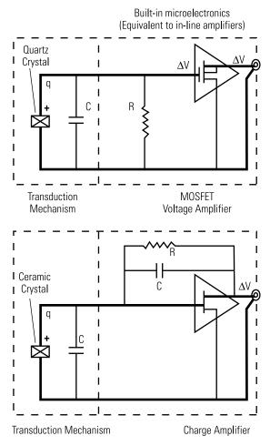
Figure 4. Basic Quartz and Ceramic ICP® Sensors
