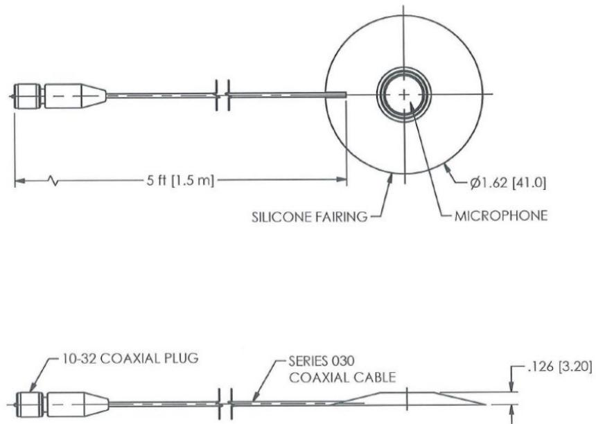
Figure 1 Surface microphone size
