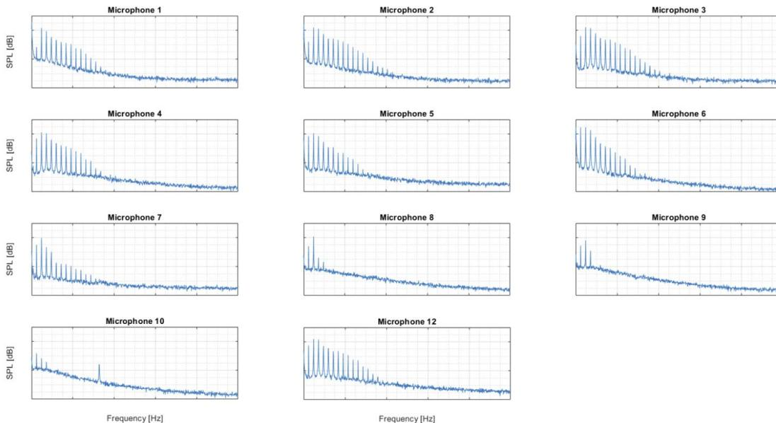
Figure 6 SPL Spectral shape for each external microphone, 175 kts
