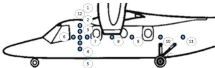
Figure 2 Layout diagram of external microphones
