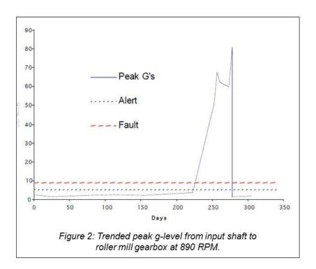
The PeakVue<sup>™</sup> spectral data (computed from the PeakVue<sup>™</sup> time data presented in Figure 1) positively identified the fault as an inner race fault. Based on the peak g-levels, a decision was made to replace the bearing around day 275 in Figure 2 (g-levels around 80 g's). The peak g level returned well below the alert level (see Figure 2) post bearing replacement. A picture of the removed bearing showing the inner race fault is presented in Figure 3.
