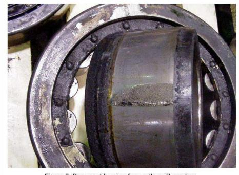
Figure 3: Damaged bearing from roller mill gearbox.
