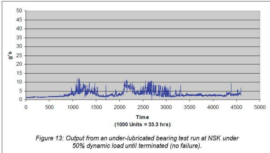
*Figure 13: Output from an under-lubricated bearing test run at NSK under 50% dynamic load until terminated (no failure).*
