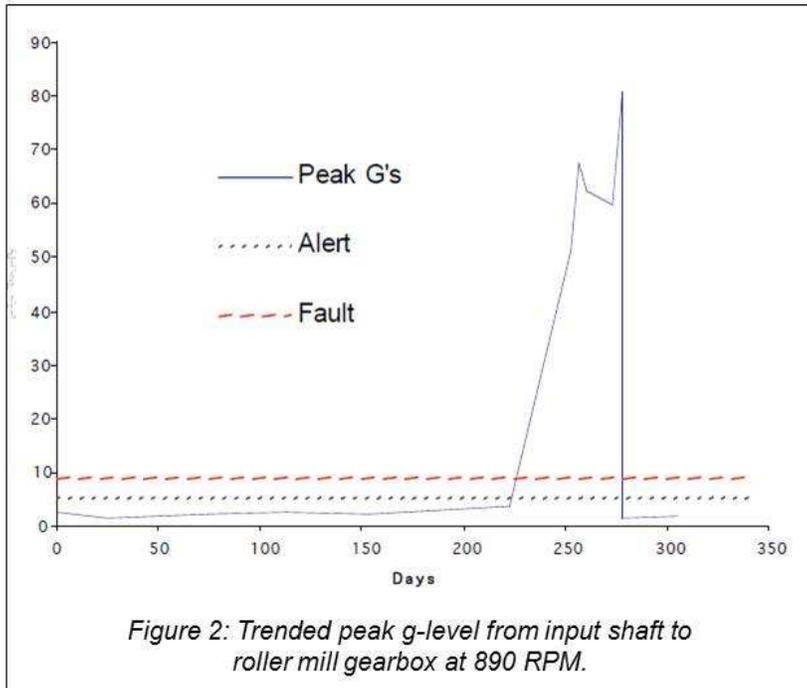
The PeakVue™ spectral data (computed from the PeakVue™ time data presented in Figure 1) positively identified the fault as an inner race fault. Based on the peak g-levels, a decision was made to replace the bearing around day 275 in Figure 2 (g-levels around 80 g's). The peak g level returned well below the alert level (see Figure 2) post bearing replacement. A picture of the removed bearing showing the inner race fault is presented in Figure 3.
