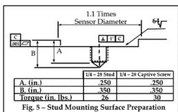
One last point worth noting regarding mounting involves surface preparation. In addition to surfaces being as flat as possible, clean and free of debris, and the mounting holes to be perpendicular, the mounting surfaces should be lightly coated with a lubricant. This coating aids in the transmissibility of the higher frequency vibrations and improves high frequency response of sensors. Silicone vacuum grease, heavy machine oil, or bees wax are commonly used.
