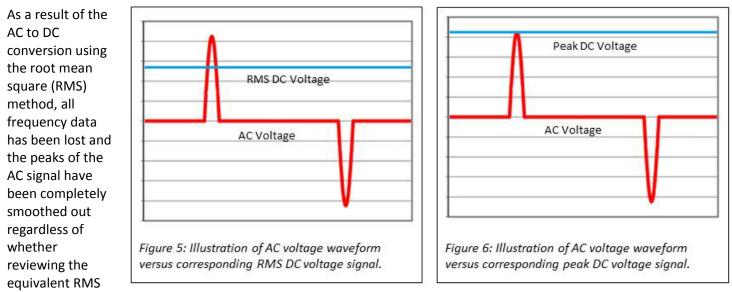
or peak DC voltage (and subsequently current) signal. This makes the resulting 4-20 mA signal ideal for long-term process monitoring but not for in-depth analysis. See Figure 5 and 6 for illustrations.
