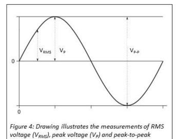
voltage (V<sub>P-P</sub>) on an AC voltage waveform.
