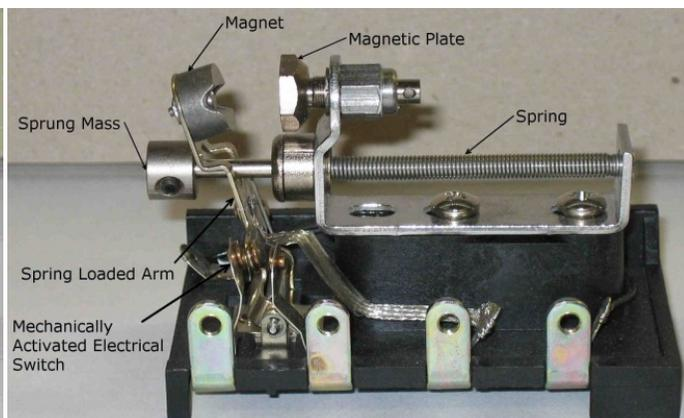
Figure 6: Tripped mechanical switch mechanism with labeled parts
