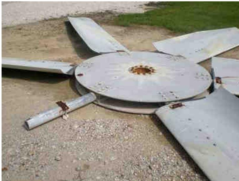
Figure 1: Catastrophic failure of a large fan due to high vibration
