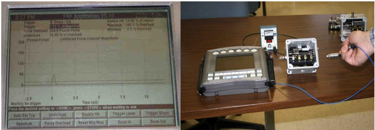
Figure 8: Impact test for mechanical vibration switches
