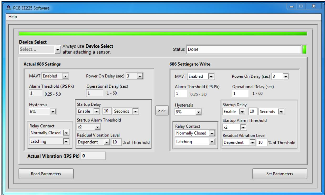
Figure 10: Programming screen for USB programmable electronic vibration switch
