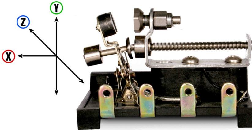
Figure 7: The sprung mass is sensitive to motion in three axes.
