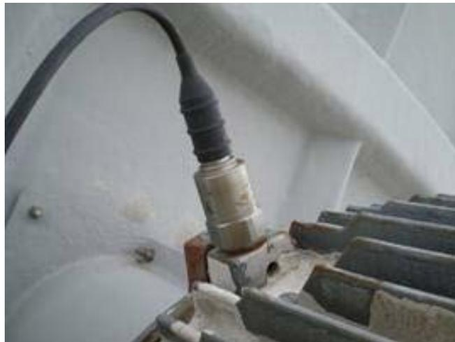
Figure 4: IMI USB Programmable Smart Vibration Switch mounted on a motor
