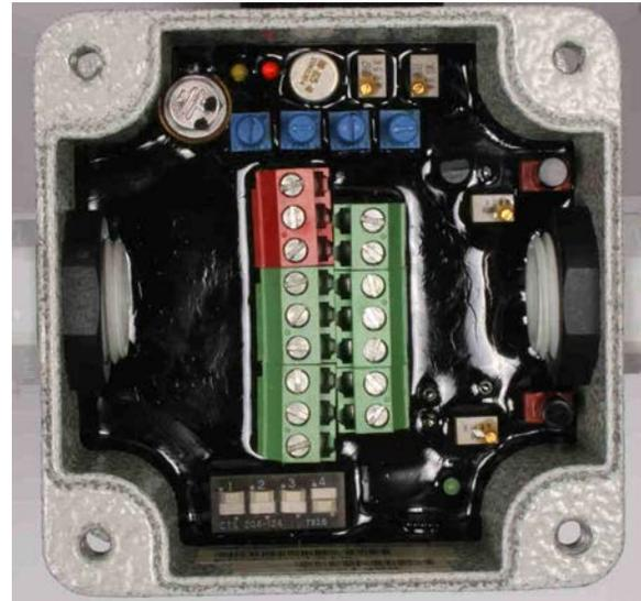
Figure 3: Traditional IMI Electronic Vibration Switch
