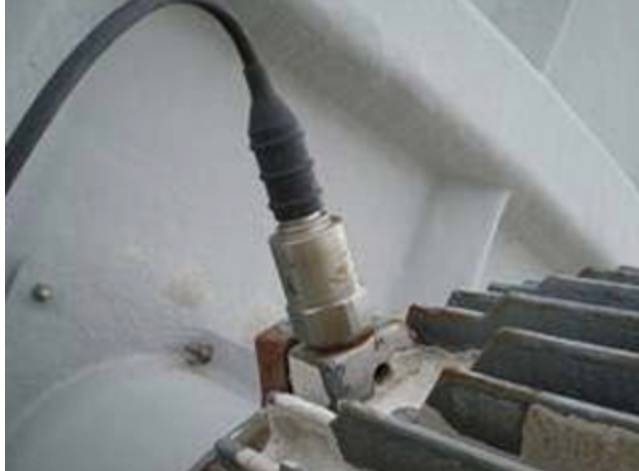
Figure 5: IMI USB-Programmable Smart Vibration Switch mounted on a motor.
