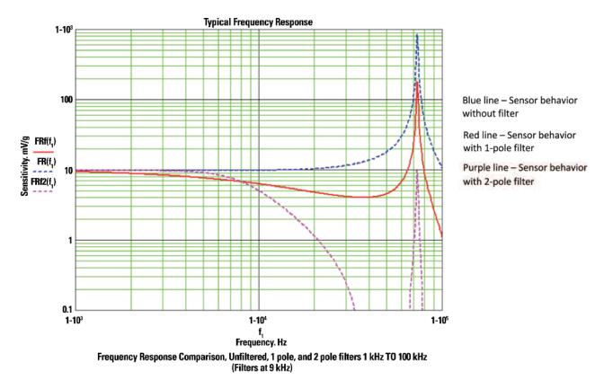
Figure 3 – Unfiltered and Filtered Sensor Response
