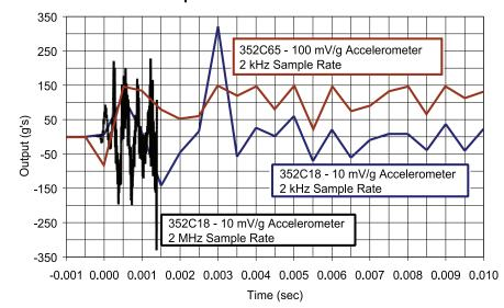
Sample Rates - 2MHz vs. 2kHz
