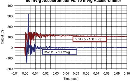
100 mV/g Accelerometer vs. 10 mV/g Accelerometer
