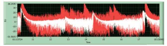
Figure 2 – Saturated amplifier example #2
