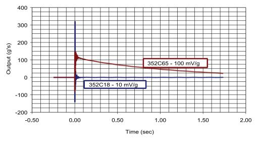
100 mV/g Accelerometer vs. 10 mV/g Accelerometer
