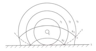
Figure 3: Strong Shock Wave Interaction with a Reflective Surface
