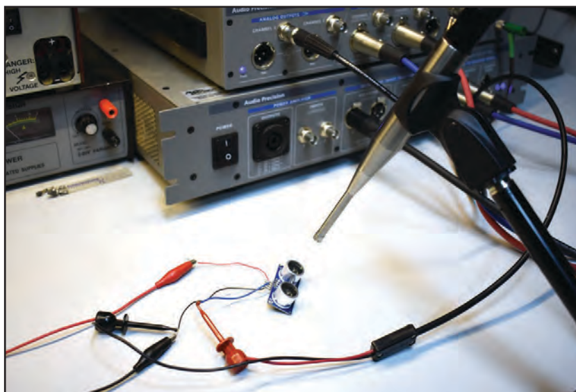
Photo 2: The 376A31 mic was used to measure the output of a popular ultrasonic transducer module. (Photo by Cynthia Wenslow)
