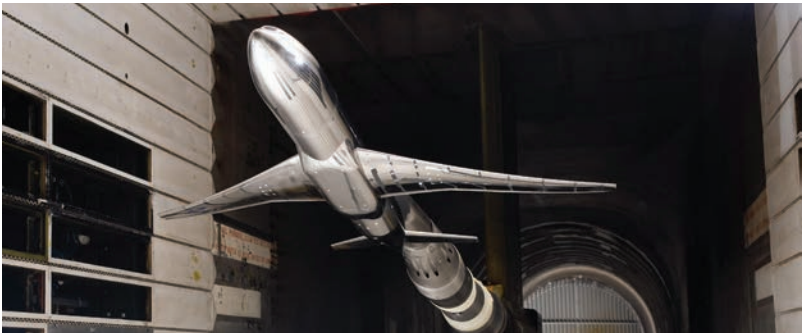
Figure 32: Aircraft model mounted in a wind tunnel for aerodynamic and aeroacoustic testing.
