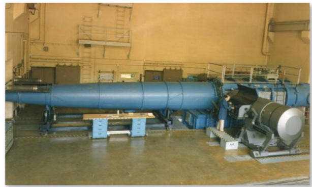
Figure 45: Overview schematic of Tunnel 9 showing nozzle and test cell configuration.
