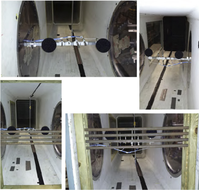
Figure 43: Microphone mounting configurations: head-on (left) and parallel (right) orientations, with (lower) and without (upper) turbulence generators. Flow direction is into the page.
