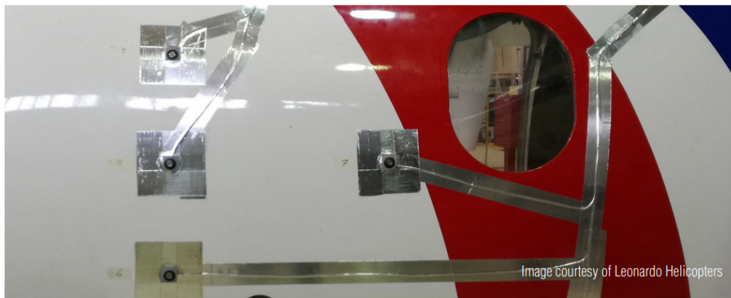
Figure 54: Photograph of external microphone installation on tiltrotor aircraft (courtesy of Leonardo Helicopters).
