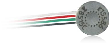
Figure 25: Endevco Model 8515C is used for surface-mount applications and measures 6.33 mm in diameter and 0.76 mm thick.
