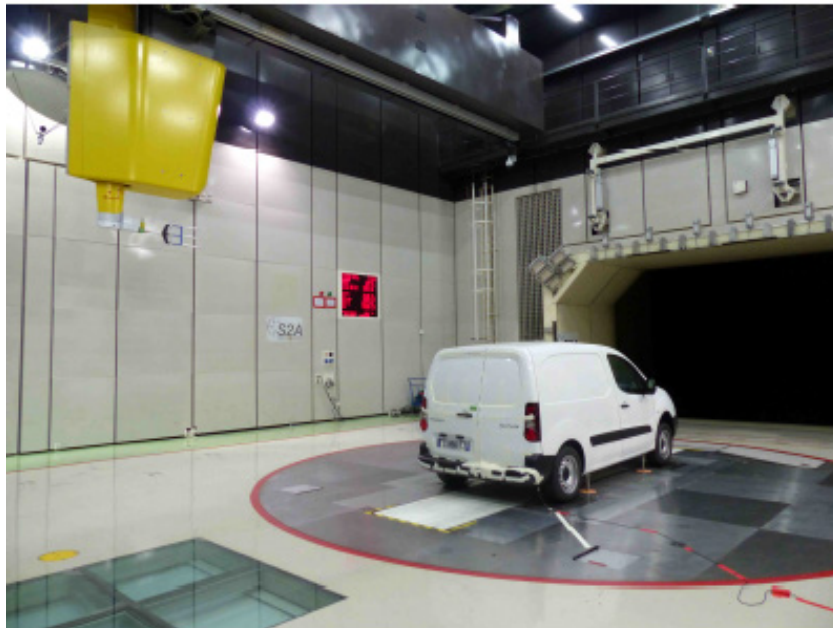
Figure 30: Van tested in a partially guided (plenum) test section of the GIE-S2A semi-acoustic automotive wind tunnel [2].
