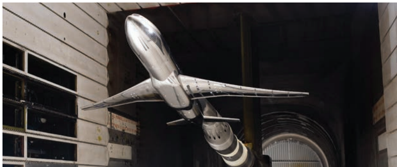
Figure 32: Aircraft model mounted in a wind tunnel for aerodynamic and aeroacoustic testing.
