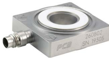
Figure 10: PCB Model 260B02 is an ICP® triaxial force ring sensor capable of measuring forces along three orthogonal axes. Requires external preload with mounting stud.
