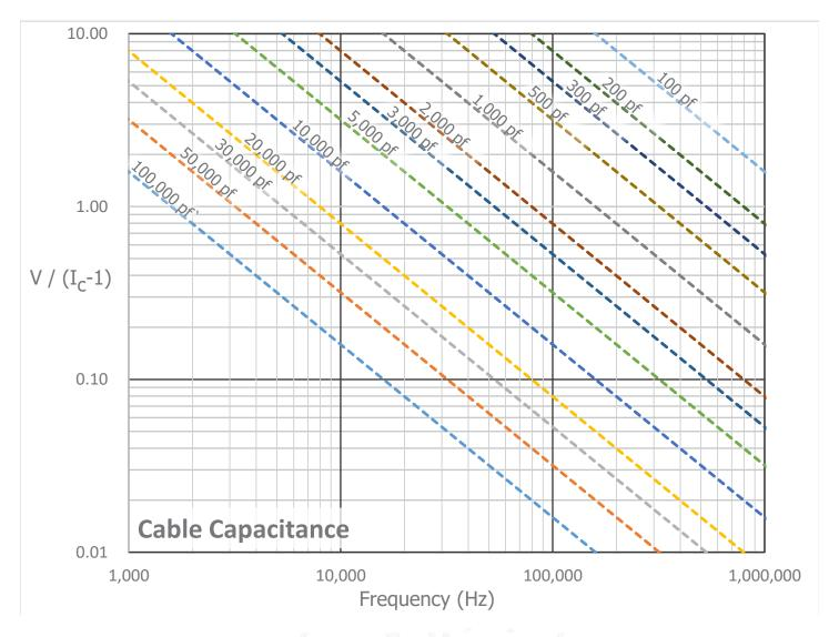
Figure 4: Cable Driving Nomograph
