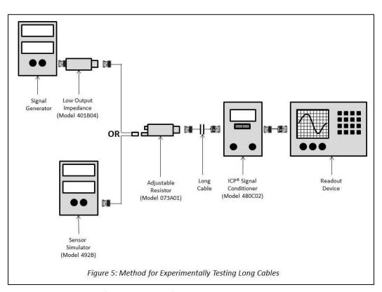
the expected measurement signal. Observe the ratio of the amplitude from the signal generator or sensor simulator to that shown on the readout device.
