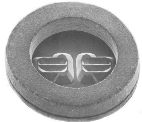
Figure 3 – Photograph of diaphragm, glass-bonded to heavy silicon ring, 0.1 in (2.5 mm) O.D. > by 0.02 in (0.5 mm) thick.
