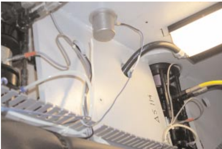
PCB Series 393 Accelerometer Typical Mounting Location Inside Main Weldment
