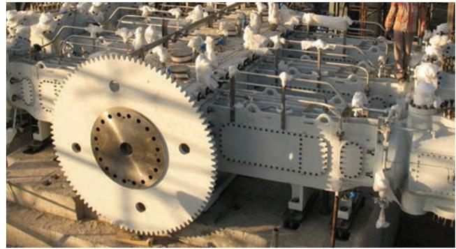
Reciprocating compressors can develop devastating faults in a short period of time. Mechanical looseness caused by a cracked rod nut, loose bolt, or excessive clearance can deteriorate quickly resulting in catastrophic failure of the compressor. In extreme cases, this can happen in a matter of minutes.
