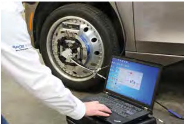
TOP: Swift Evo units are subject to a highly refined, automated process that calibrates the entire transducer assembly, cycling through each channel while simultaneously exciting all other channels
