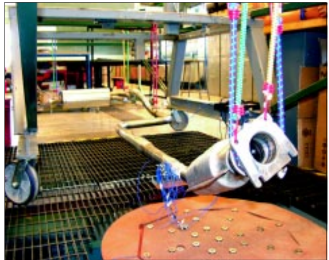
Figure 4. Photo of exhaust subsystem under investigation supported with elastic cords to approximate free-free boundary conditions.
