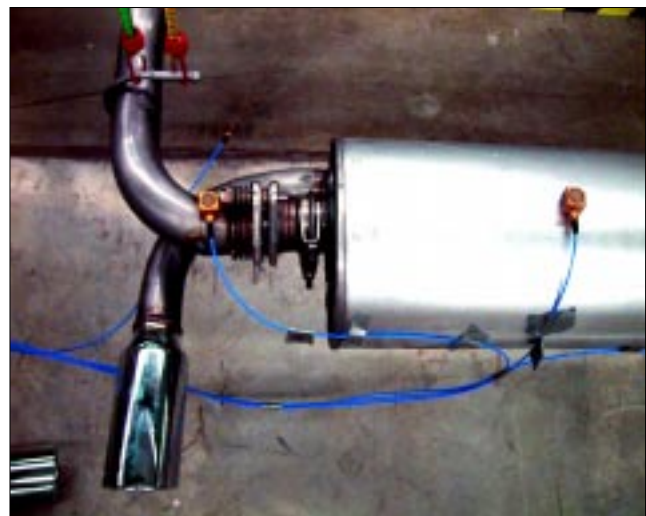
Figure 10. Photo of inlet pipe of muffler fitted with Metex joint for reducing the exhaust torsional coupling stiffness at that location to mitigate the vibration problem.
