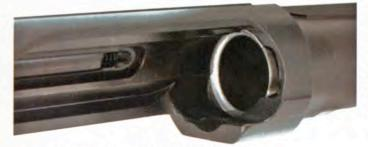
One part of the Super Black Eagle's unique operating system is a rotating bolt with two lugs that engage cutouts in the steel barrel extension.
