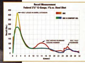
In determining how to address the problem of perceived recoil, **Benelli engineers designed** unique test equipment to evaluate how recoil was delivered to the shooter. Benelli claims that the ComforTech System reduces felt recoil by a measurable amount over comparable shotguns.
