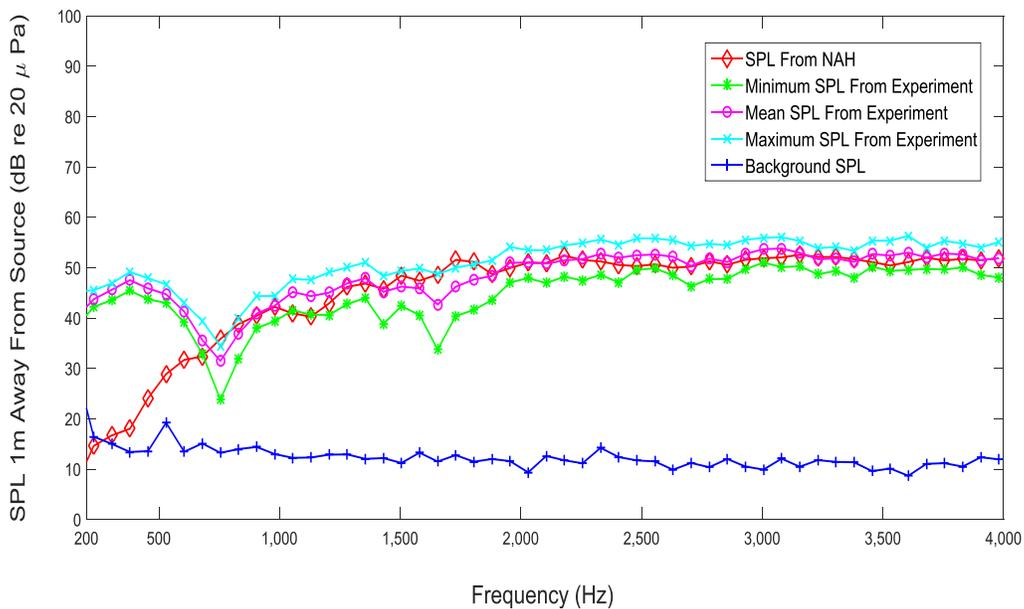
Comparison of experimental and analytical pressure distribution 1m away from source
