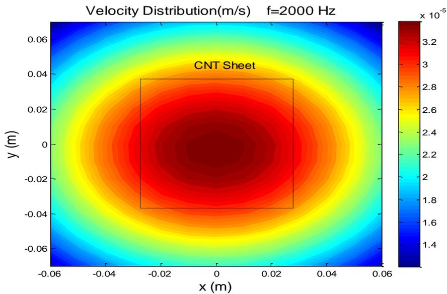
These velocity distributions were measured over a frequency range of 200 Hz to 4 kHz. The velocity variation over the source surface was calculated and is shown below. It was found that as frequency increases, the surface particle velocity variation also increases proportionally.
