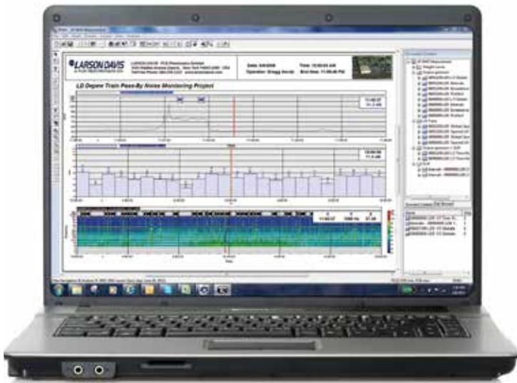
The Model 831 can be used to record the evolution of sound pressure level over time as a Time History (TH). The Time History is then used to profile the observation period, which can vary from a couple of seconds to continuous monitoring.
