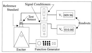
Figure 10. Typical Back-to-Back Calibration System
