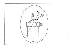
Figure 15. Mounting Triaxial Sensors (Incorrect)
