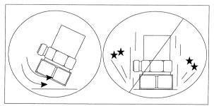
Figure 7. Magnet Mounting
