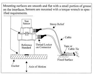
Figure 12. Typical Calibration Set-Up
