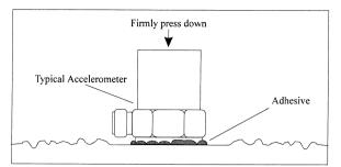
Figure 5. Direct Adhesive Mounting
