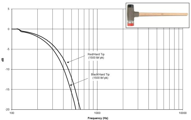
Hammer model selection involves determining the size and mass of the hammer structure which will provide the force amplitude and frequency content required for proper excitation of the structure under test. Large, heavy structures like locomotive frames, tanks and bridges require an instrumented sledgehammer; small structures like compressor blades often require mini-hammers. Some very large structures may require a massive mechanical ram instrumented with a force-sensing impact head.
