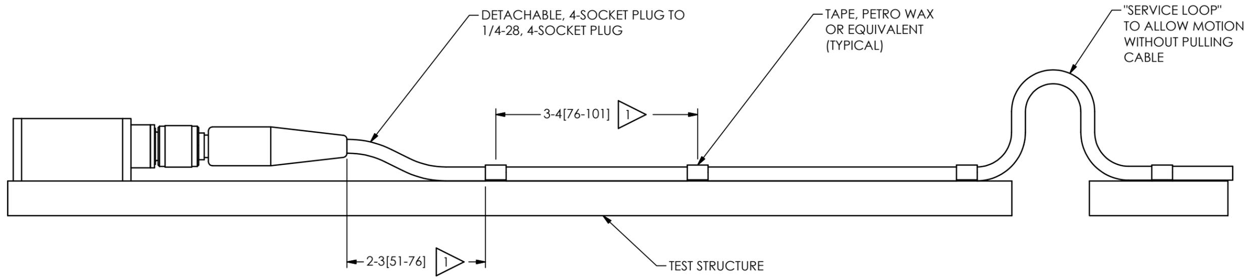
1 FASTEN CABLE TO TEST STRUCTURE TYPICALLY WITHIN 2-3" [51-76] OF SENSOR. THEN FASTEN AGAIN WITHIN 3-4" [76-101] OF PREVIOUS ATTACHMENT. BETWEEN THE TEST STRUCTURE AND A FIXED STRUCTURE, ALLOW A SERVICE LOOP LARGE ENOUGH TO PREVENT PULLING OF THE CABLE WHEN SHAKING. MORE ATTACHMENT POINTS WILL PROVIDE LESS NOISE IN THE RESULTING DATA. LOOSE CABLES OR PARTS ELSEWHERE ON THE TEST STRUCTURE CAN ALSO GENERATE "NOISE" ON THE SIGNAL RECEIVED FROM THE MODEL 3711 SERIES.
