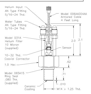
**123** Series: Water- Cooled & Helium Bleed Rocket Motor, ICP<sup>®</sup> and Charge Sensors
