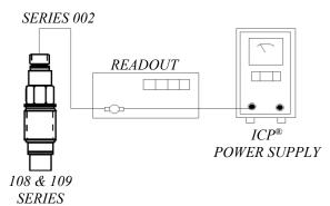
With this arrangement, the readout is direct-coupled to the sensor and the output signal will be added to the DC bias voltage (11 VDC nominal).
