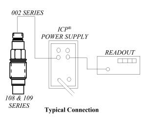
The figure above shows the 108 & 109 Series connected to a PCB Model 484B06 power unit. The 484B06 is a power unit that can be AC or DC-coupled.
