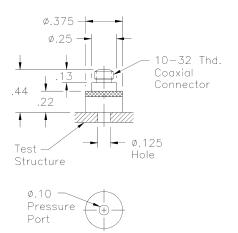
Models 103A02 and 103A12: ICP<sup>®</sup> Sound Pressure Sensors
