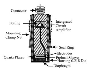
Typical ICP® Probe Style Sensor
