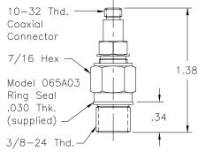
**Model 102A05 Thread Mount Design, Ground-Isolated Sensor**
