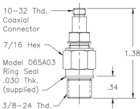
**Series 102: Thread Mount Design, Ground-Isolated Sensor**
