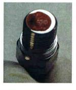
Wear a rubber glove and force sealant between probe and mounting location or adaptor with finger.
