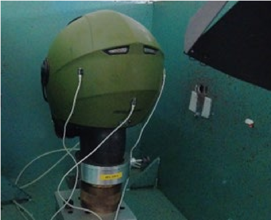
Picture 3: Test set-up for metallic ball impact on rear of helmet
