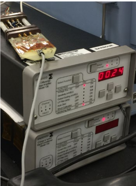
Picture 7: One end of the cable is attached to a dummy Wheatstone bridge. The bridge is powered via a signal conditioner
