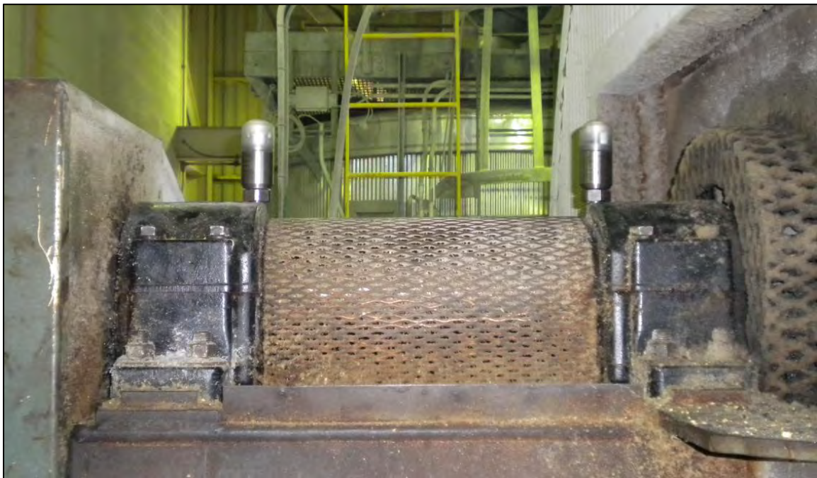
Figure 4 – Echo® Wireless Sensors Mounted on Recirculating Fan Bearings
