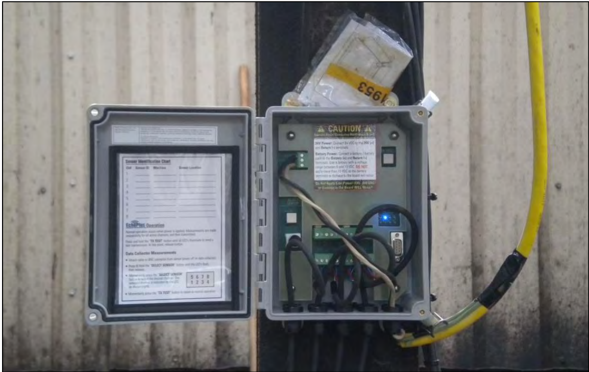
Figure 3 – EchoPlus® Measuring One of Eight Connected Accelerometers
