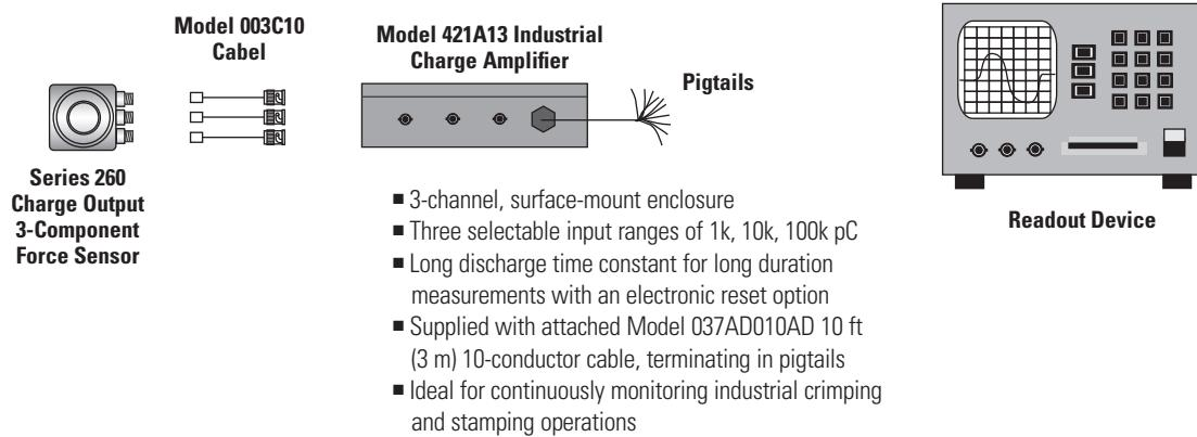
Figure 12. Low-cost System Utilizing 3-Channel Industrial Charge Amplifier
