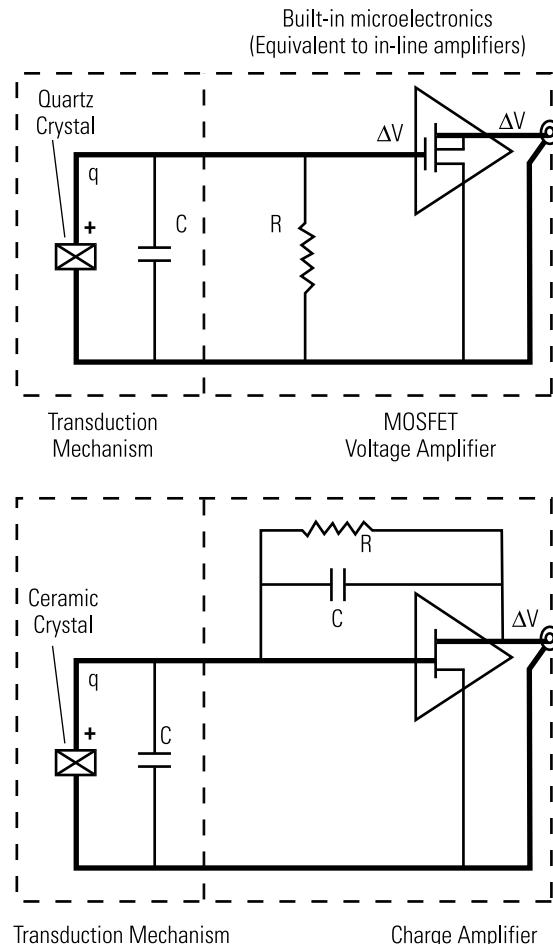
**Figure 4. Basic Quartz and Ceramic ICP® Sensors**
