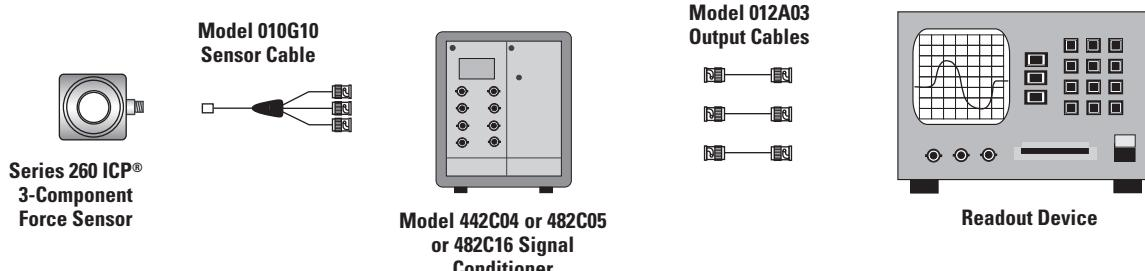
Figure 11. System Utilizing a ICP® Sensor Signal Conditioner
