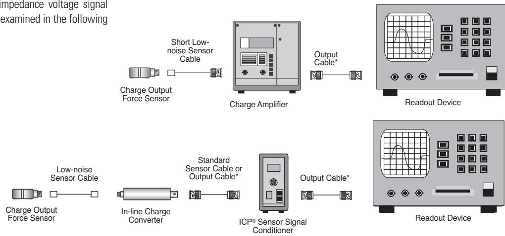
A fixed in-line charge converter may be utilized to simplify setup or to make use of an existing ICP® sensor signal conditioner.
