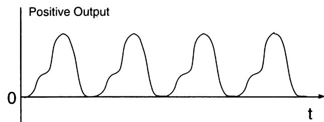
Figure 10. Positive Polarity, Zero-based AC Output
