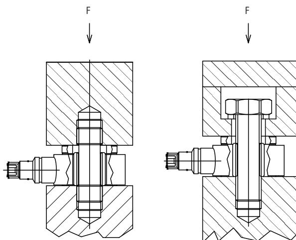
Figure 8. Force Ring Sensor Installations
