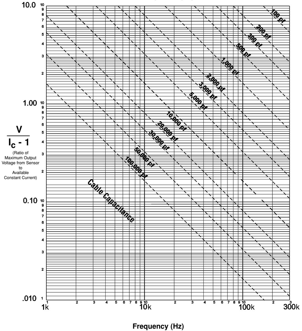
$f_{max}$  = Maximum frequency given the following characteristics
