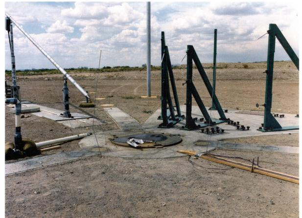
A typical blast sensor installation requires long cables for signal transmission. Data acquisition equipment may be thousands of feet away.
