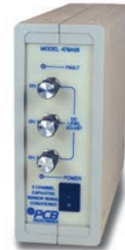
Model 478B05 3-channel unity gain 36 VDC powered optional external battery pack
