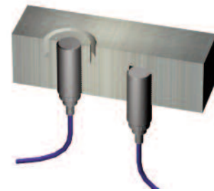
Figure 11: Strain Isolated Pressure Transducer Left – Isolated “Check” Transducer Right
