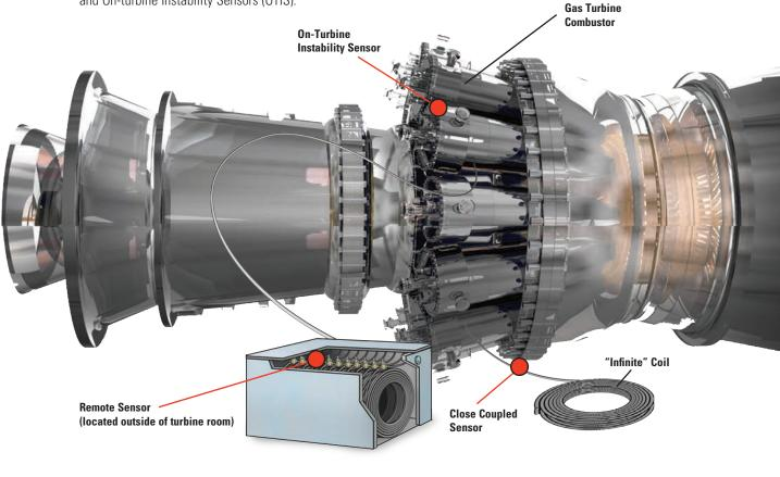
The diagram above shows a typical setting for a gas turbine in a power generation plant. Shown within the illustration are the three standard methods of measuring pressure; Remote, Close Coupled and On-Turbine Instability Sensor (OTIS). The red bullets indicate the location of the actual sensor for each different method.
