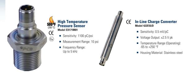
Close coupled sensors permanently mounted to a gas turbine are ideal for monitoring combustion dynamics (instability). Operating at a wider frequency range than remote sensors, the high sensitivity and higher-temperature capability of these sensors allow for precision measurement in turbine locations where the application of other instrumentation is not possible.
